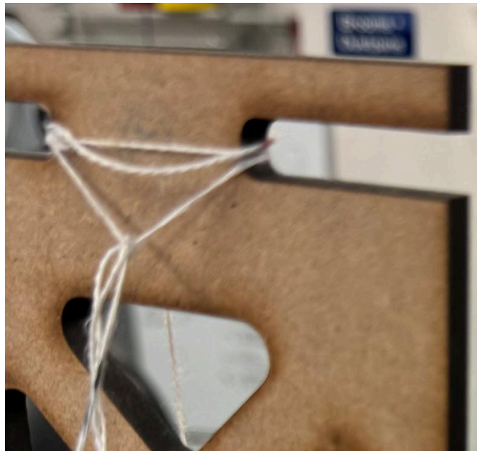
Figure 16: Twine loosely looped around laser cut attachment point
